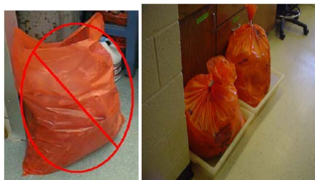
Figure 6 - Proper location of contaminated materials
